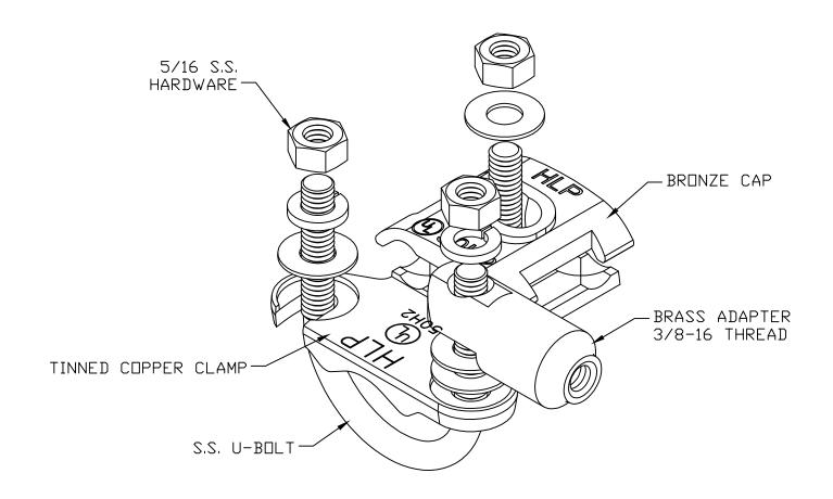
CLAMP RANGE 0.840 THRU 1.315" D.D. 1/2-1 IN. NOM. PIPE BASE FOR 1/2 IN. AIR TERMINAL
