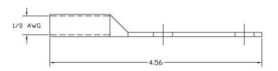
SEAMLESS COPPER TUBING. 122 ALLOY SOFT COPPER. TIN PLATED
