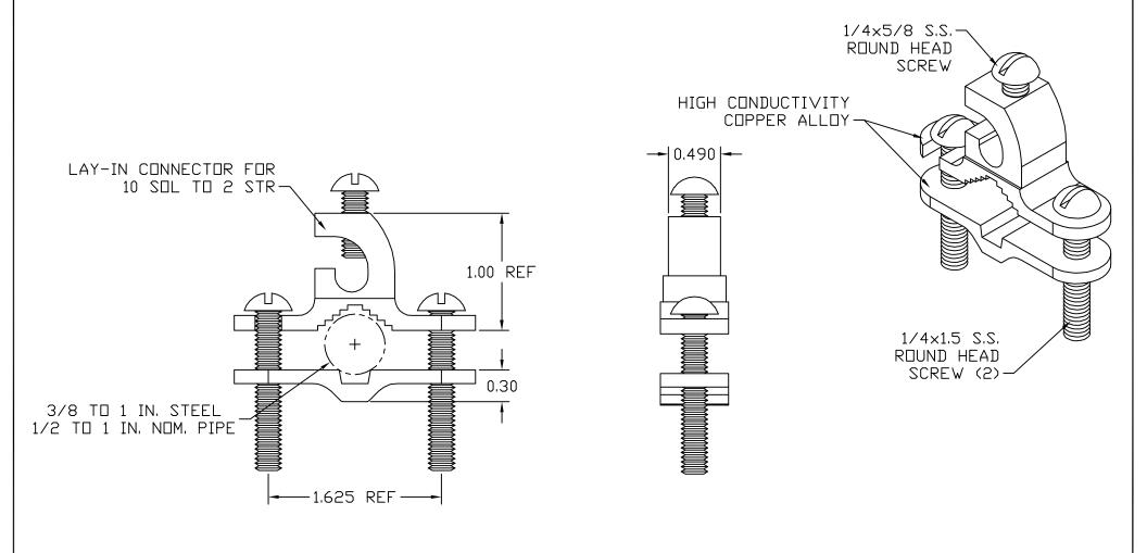
SUITABLE FOR DIRECT BURIAL IN EARTH AND CONCRETE
