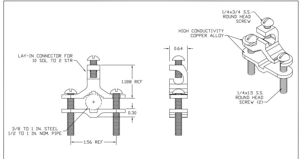
SUITABLE FOR DIRECT BURIAL IN EARTH AND CONCRETE
