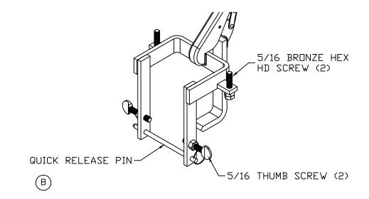
NOTES: 1. CLEAN AND REMOVE ALL GRIT PRIOR TO FINISHING. 2. BLUE PAINT FINISH ON PLAIN STEEL ITEMS AFTER WELDING, BEFORE FINAL ASSEMBLY.
