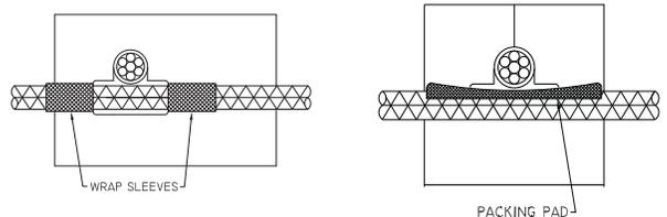
*Note: Wrap Sleeve MUST go all the way around the rebar.*
