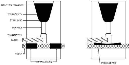
*Note: Wrap Sleeve MUST go all the way around the rebar.*
