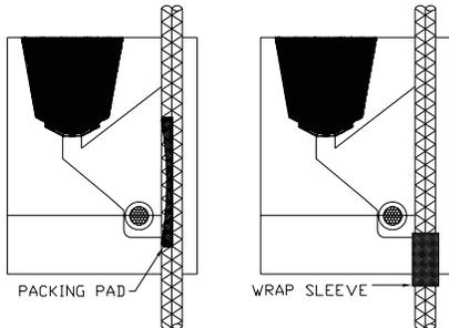
*Note: Wrap Sleeve MUST go all the way around the rebar.*
