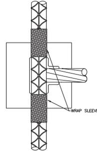
*Note: Wrap Sleeve MUST go all the way around the rebar.*
