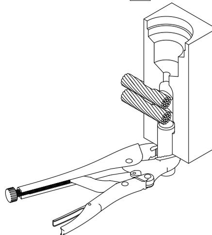
**Place the end of both cables under the center of the tap hole. The bottom cable must sit on top of ground rod. Use locking pliers or a clamp on the rod below the mold to prevent it from slipping when the mold is fired.**
