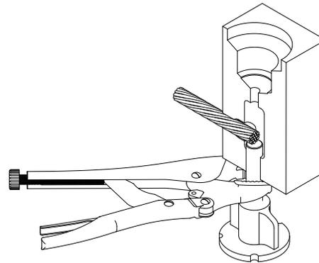
**Place end of cable under the center of the tap hole. Cable must sit on top of earth boss. Use locking pliers or a clamp on the earth boss below the mold to prevent it from slipping when the mold is fired.**
