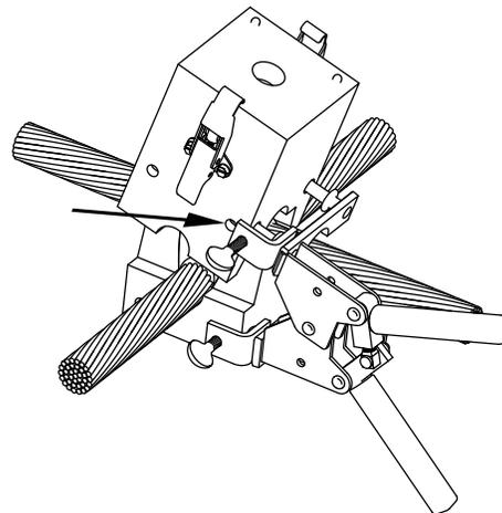
**Place tap cable over run cable. Cables are uncut. To remove mold more easily from finished weld: unscrew top thumbscrew of mold handle. Re-fasten mold handle thumbscrew prior to next connection.**
