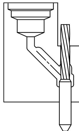
**For cables larger than 4/0, place end of ground rod to bottom of tap hole. Butt cable against top of ground rod.**
