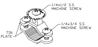
1/2" THRU 3/4" CONDUIT CLAMP CAST COPPER TIN PLATED
